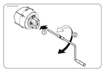
The crank can be mounted to the drive unit after usage.
